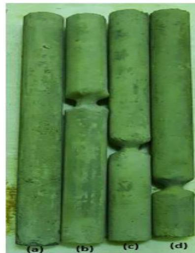
**Figure 3.** Model piles with different positions of neck.
