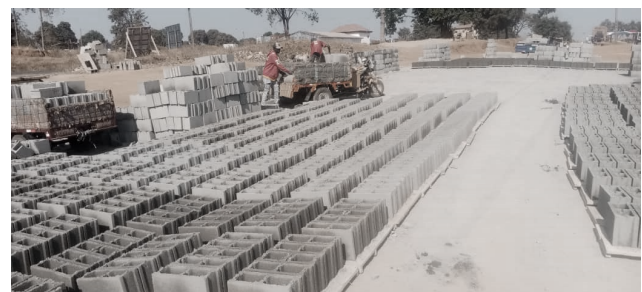
Figure 14. Blocks made with mixtures (pozzolan-cement) in the locality.
