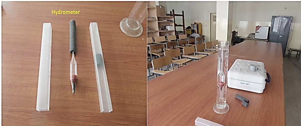
Figure 11. Device (tool) of the hydrometer for determination of soil mechanical analysis.
