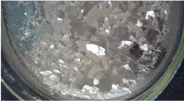
Figure 7. This is a "cracked" film, into which the drying collagen solution, prepared in water with a potential of +250 mV, has turned. Water used had 20 – 22 °C.
