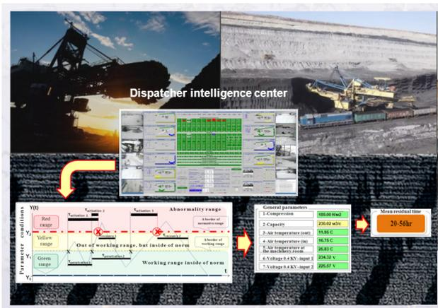
Figure 14. Example of a prognosed residual time before the next parameter abnormality
