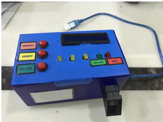
**Figure 16.** Final Prototype of the Fingerprint School Debit Transaction System (Fingerprint Collection Module)
