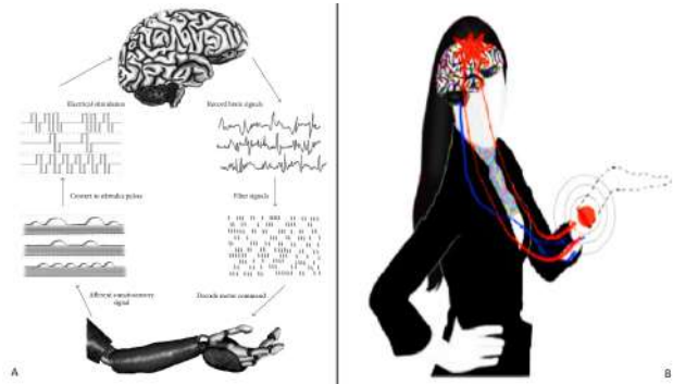
Figure 7. Working of neural prosthetics using a brain-machine interface (a). Phantom limb pain depiction (b)
