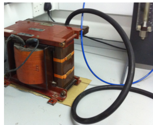
Figure 4. Transformer 2, 1:50 up to 12000V
