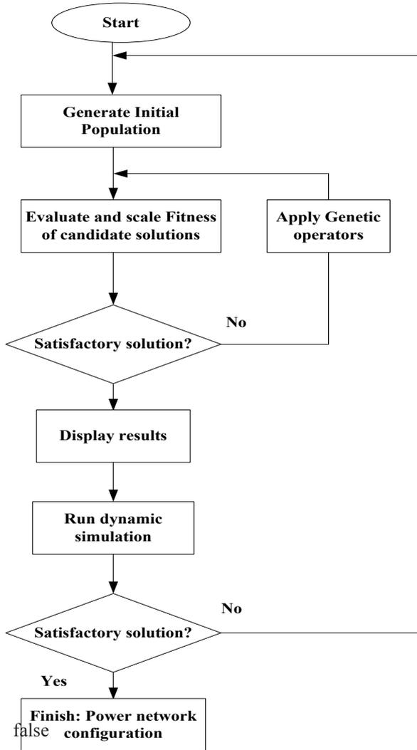
Figure 4. Flowchart of GA for optimal allocate of compensator resources
