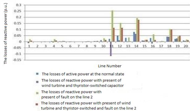
Figure 10. Lines' reactive power losses with wind farm and TSSC and short circuit in line 6-12
