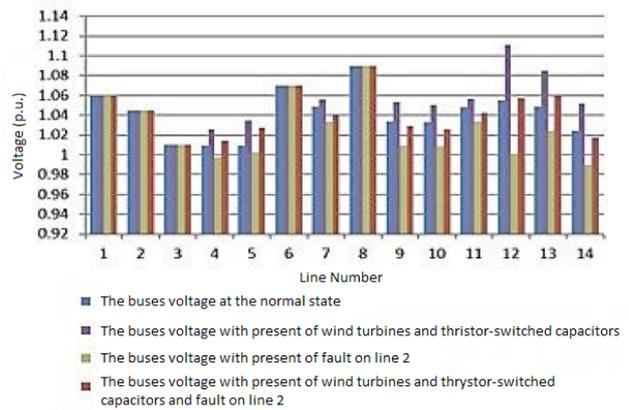
Figure 8. Comparison of bus voltage with/without wind farm and TSSC and short circuit in line 6-12
