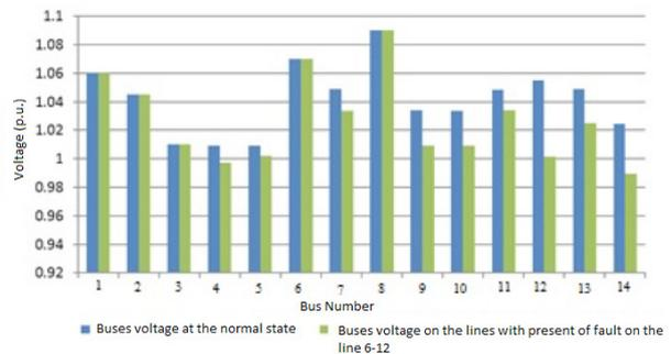
Figure 5. Bus voltages with short circuit in line 6-12
