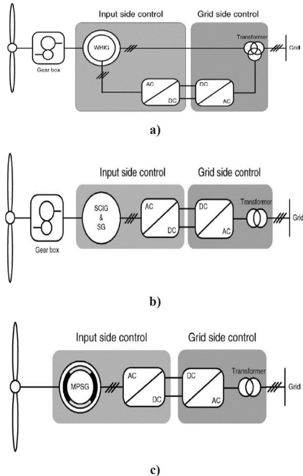
Figure 3. Topology of connected wind turbines to grid [1]
