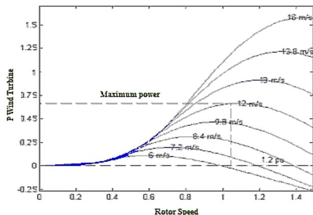
Figure 2. Mechanical Power of Wind Turbine against various wind speeds<sup>[1]</sup>
