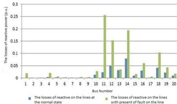
Figure 7. Lines' reactive power with short circuit in line 6-12
