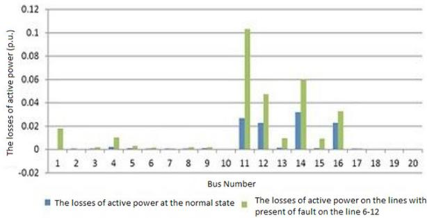
Figure 6. Lines' active power with short circuit in line 6-12
