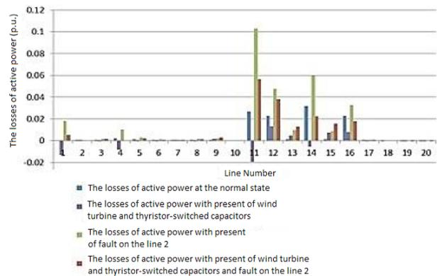
Figure 9. Lines' active power losses with/without wind farm and TSSC and short circuit in line 6-12
