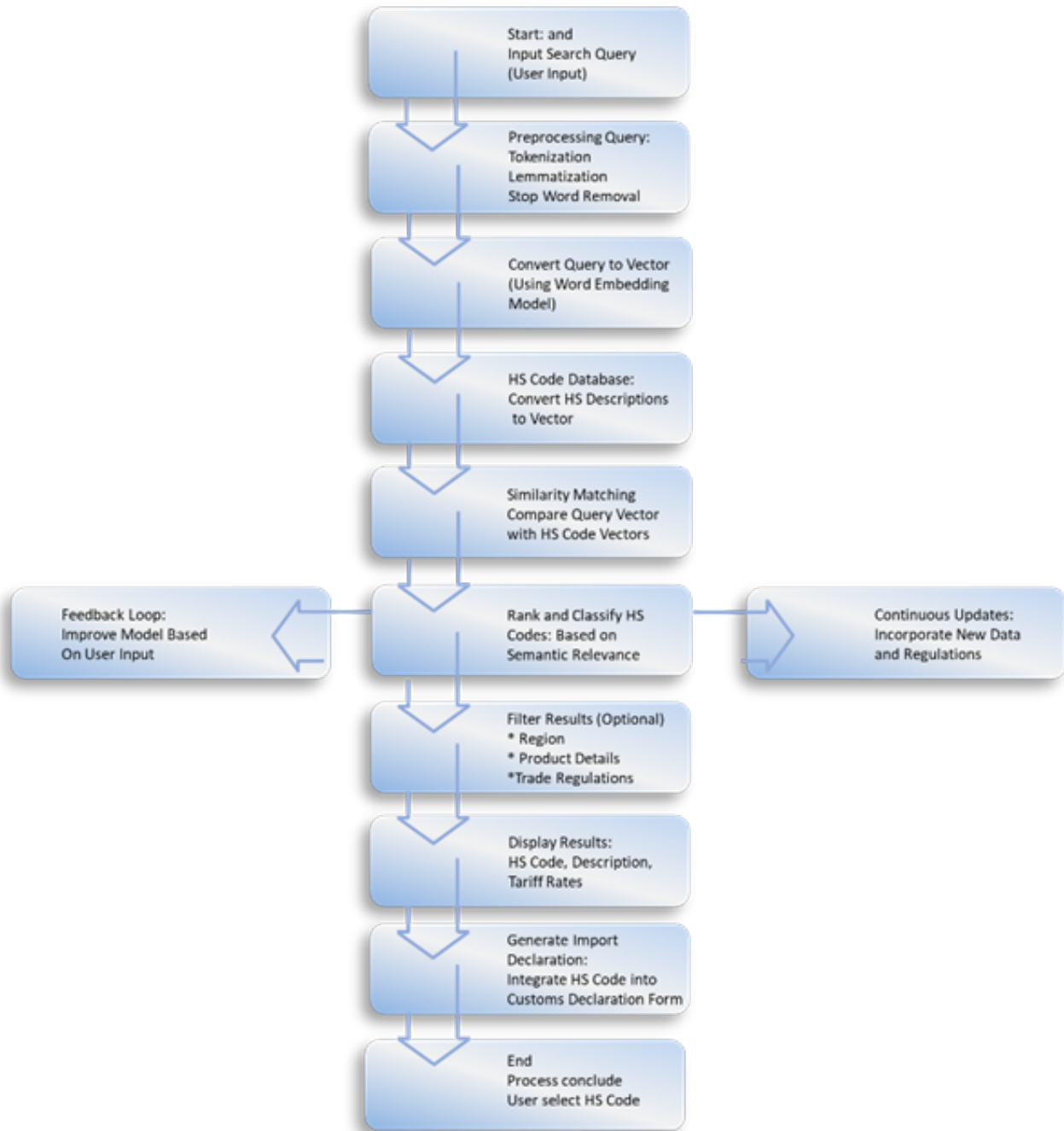
Figure 4. Full Process for HS Code Classification Using Semantic Search and Word Embeddings.
