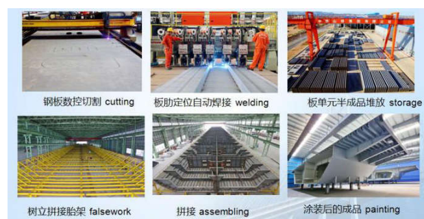
Figure 7. Production process for steel box girder
