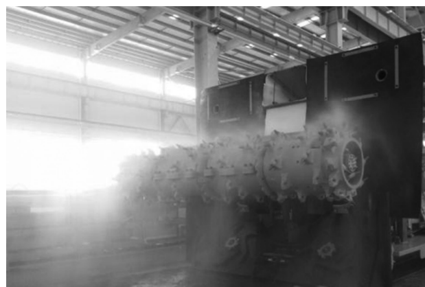
Figure 5. Semi-closed negative pressure wet type dust removal system
