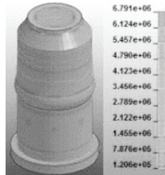
Figure 6 (e). Effective Stress Cloud Chart of Silo and Storage under 3/4 Storage
