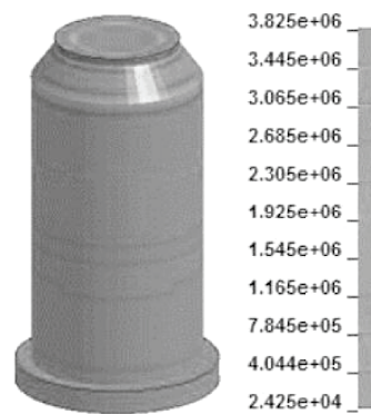
Figure 6 (a). Silo Effective Stress Cloud Chart under the Condition of Short Position
