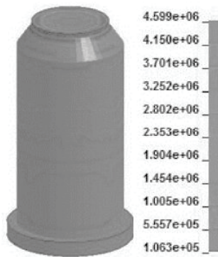
Figure 6 (c). Effective Stress Cloud Chart of Silo and Storage under 1/4 Storage
