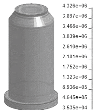
Figure 6 (b). Effective Stress Cloud Chart of Foundation under Empty Condition
