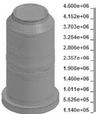
Figure 6 (d). Effective Stress Cloud Chart of Silo and Storage under 1/2 Storage
