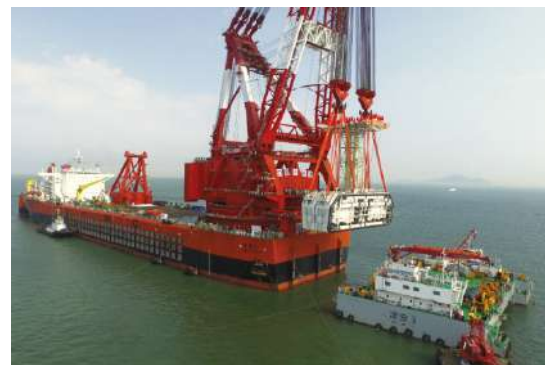
Figure 14. 12000t Floating crane for installing tunnel closure element
