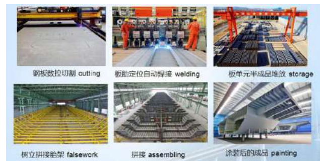
Figure 7. Production process for steel box girder
