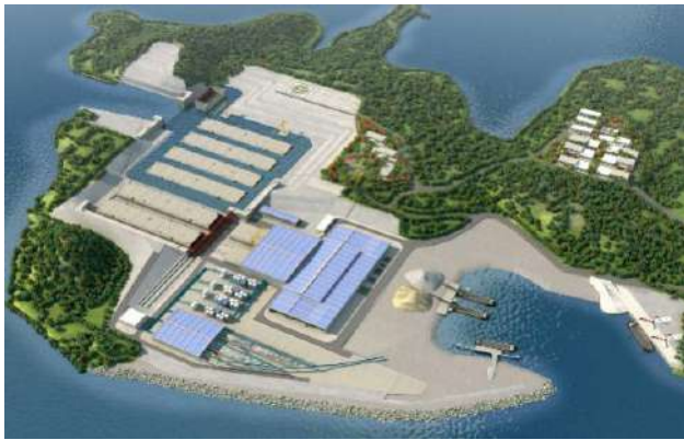
Figure 6. Layout of fabrication factory for tunnel elements
