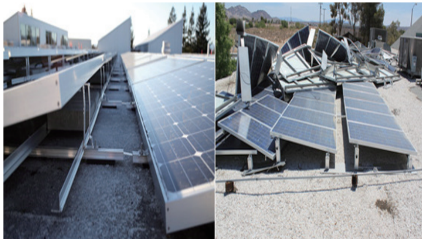
Figure 5. Failure and damage of the mount ground solar tracker caused by strong wind [37]
