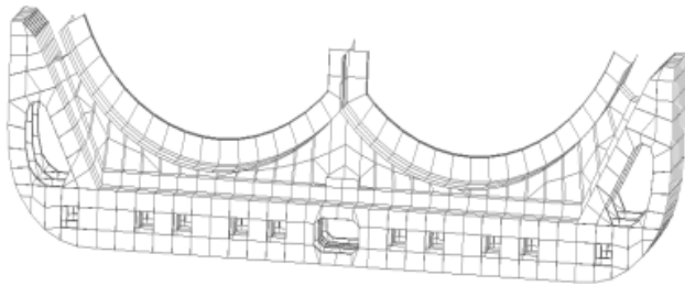
Figure 2. Temperature field analysis model of support structure in the independent LNG containment
