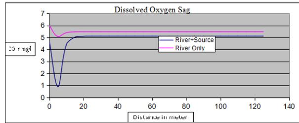
**Figure 5.** DO sag curve developed using Streeter Phelp’s model (Shiroli MIDC)
