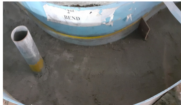
Figure 5. (Photometric view of bed, when spur dyke installed at angular displacement \theta = 0^\circ )
