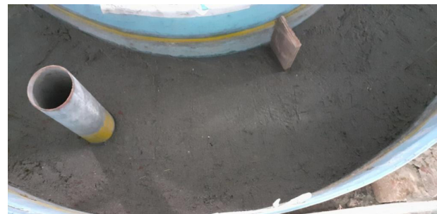
Figure 6. (Photometric view of bed, when spur dyke installed at angular displacement \theta = 20^\circ )
