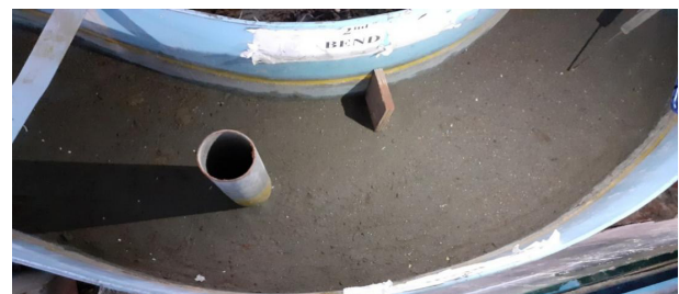
Figure 7. (Photometric view of bed, when spur dyke installed at angular displacement \theta = 40^\circ )
