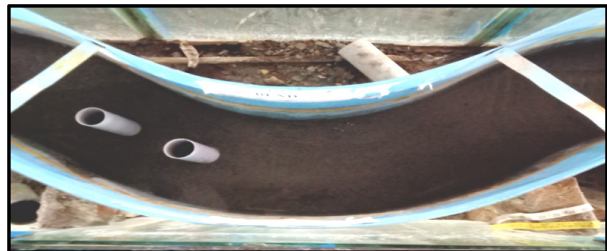
Figure 6. Showing the pier positions for 5 th Run in Bend – 2
