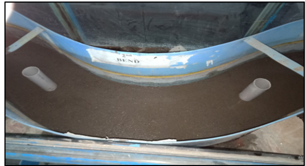
Figure 4. Showing the pier positions for 3 rd Run in Bend – 2
