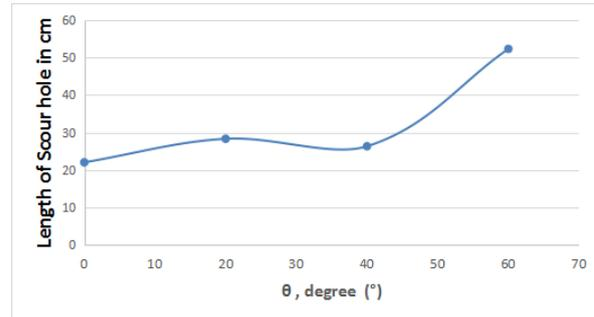
**Figure 18.** Variation of longitudinal length of scour hole of rear pier due to change in angular displacement of front pier
