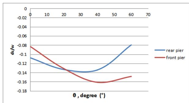
**Figure 15.** Comparison between maximum scour between rear pier and front pier at different angular displacements
