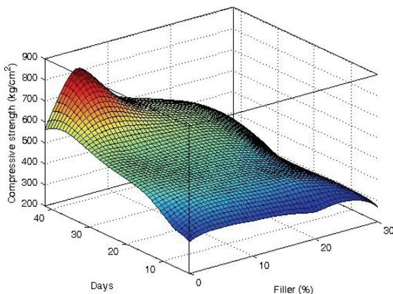
**Figure 8.** Predicted results of the comprehensive strength (kg/cm<sup>2</sup>) using ANN1
