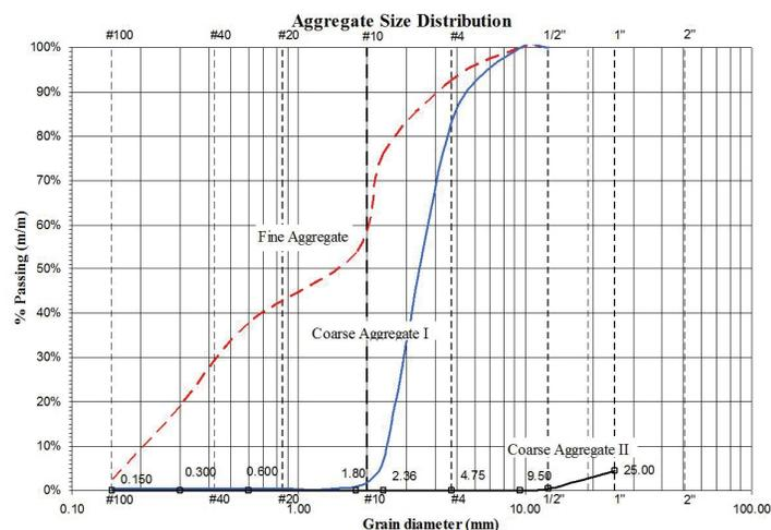
Figure 1. Sieve analysis of fine and two types of coarse aggregates
