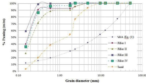
**Figure 2.** Particle Size Distribution(PSD) of fillers and sand
