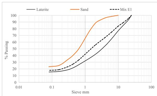
Figure 1. grading of laterite-sand-mix E1
