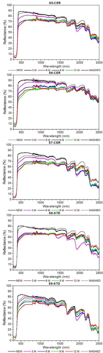
**Figure 3.** Spectral reflectance for new and aged coatings (3, 6, 9, 12 months) and after a cleaning process.
