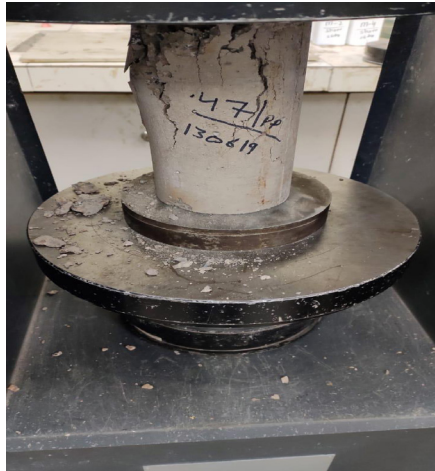
(c) NSC Cylinder with PP fiber after exposure during testing
