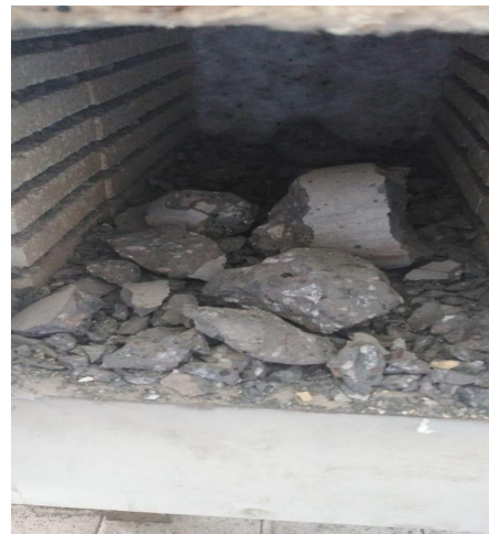
(a) Cylinder with control mix after blast in the furnace
