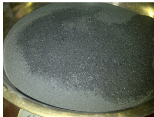
Figure 2. Palm Kernel ashes after ball-milled into finer particle
