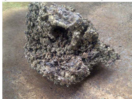
Figure 1. Palm Kernel Ashes after burning (large particle size and porous texture)
