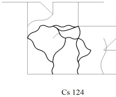
Figure 7. Typical example of loading failure
