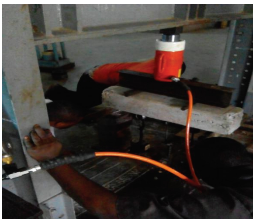
Figure 1. Flexural strength setup for beam under third-point loading
