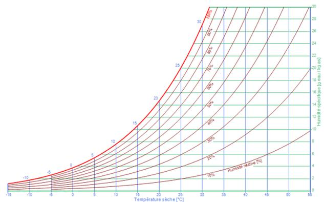
Figure 3. Air thermal process on psychrometric chart
