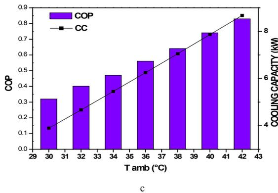
Figure 5. Influence of ambient air temperature ( $T_{amb}$ ) on: a. outlet air state from the dehumidifier, b. SHR and MRR and c. the performance of the system
