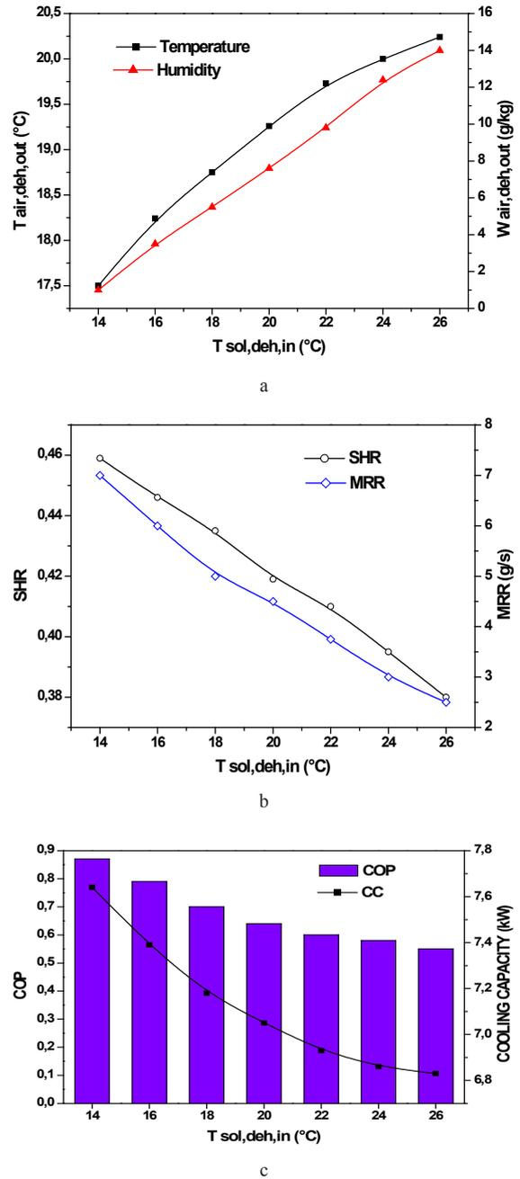
**Figure 8.** Influence of inlet desiccant solution temperature to the dehumidifier ( $T_{sol,deh,in}$ ) on: a. outlet air state from the dehumidifier, b. SHR and MRR and c. the performance of the system
