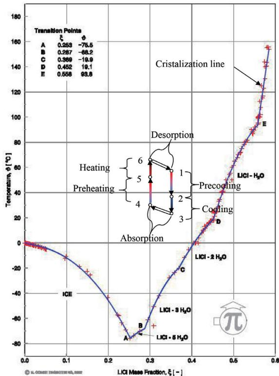
**Figure 4.** Desiccant solution cycle diagram and its process on the Conde diagram of aqueous lithium chloride solution
