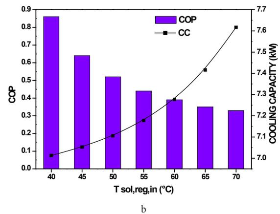
**Figure 7.** Influence of inlet desiccant solution temperature to the regenerator ( $T_{sol,reg,in}$ ) on: a. SHR and MRR and b. the performance of the system
