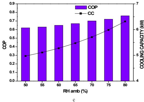
**Figure 6.** Influence of ambient air relative humidity (RHamb) on: a. outlet air state, b. SHR and MRR of the dehumidifier and c. the performance of the system
