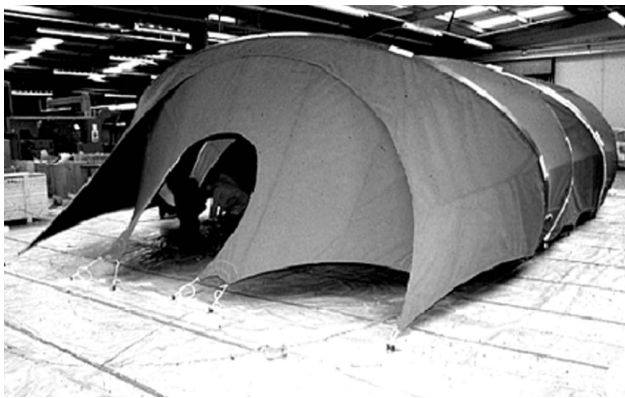
Figure 15. Revised structural configuration of full scale prototype shelter, N. K. Burford and F. W. Smith
