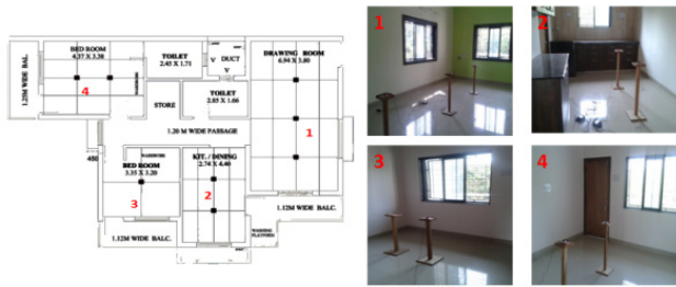
Figure 5. Plan and interior views of selected liveable spaces of dwelling units with sensors position
