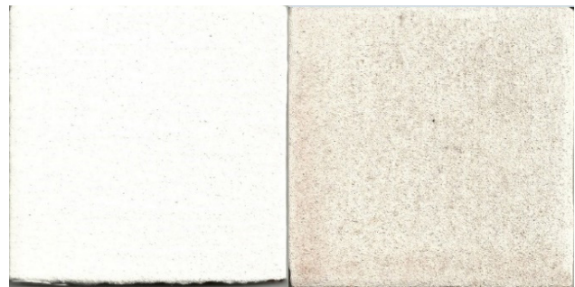
Figure 4. Sample S7-MEC, new and after 12 months of natural weathering exposure
