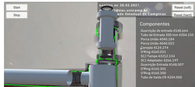
Figure 7. Exploded view superposing the real sink trap
