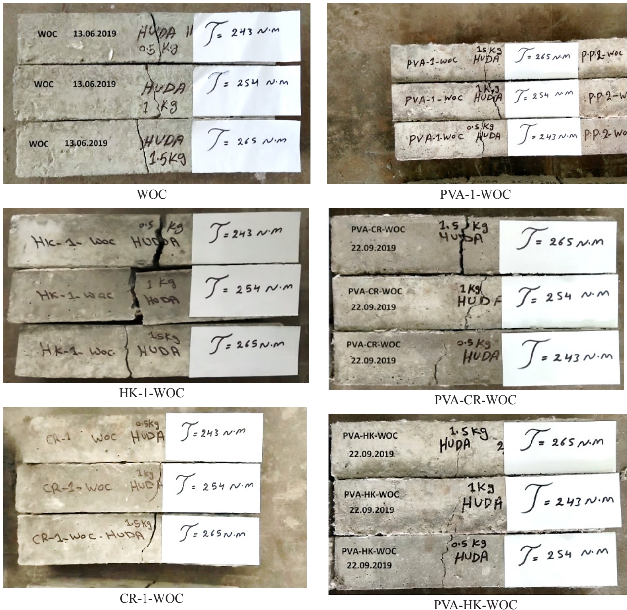
Figure 7. Combined (flexural and torsion) strength test specimens: WOC, HK-1-WOC, CR-1-WOC, PVA-1-WOC, PVA-HK-WOC and PVA-CR-WOC CR-1-WOC at failure
