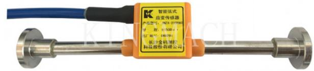
Figure 1. Picture of the JMZX-215 strain gauge
