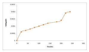
Figure 4. The generation of voltage through rice paddy straw at  $1000\Omega$  resistance
