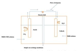
Figure 3. Dual chambered Microbial Fuel Cells (MFCs) Construction and Operation
