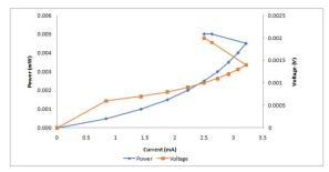
Figure 6. Polarization and power density curves through rice paddy straw
