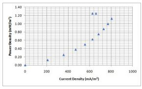
Figure 7: Power density versus Current density through rice paddy straw
