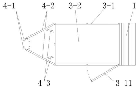
Figure 2. The overlook chart of the electric lifting table
