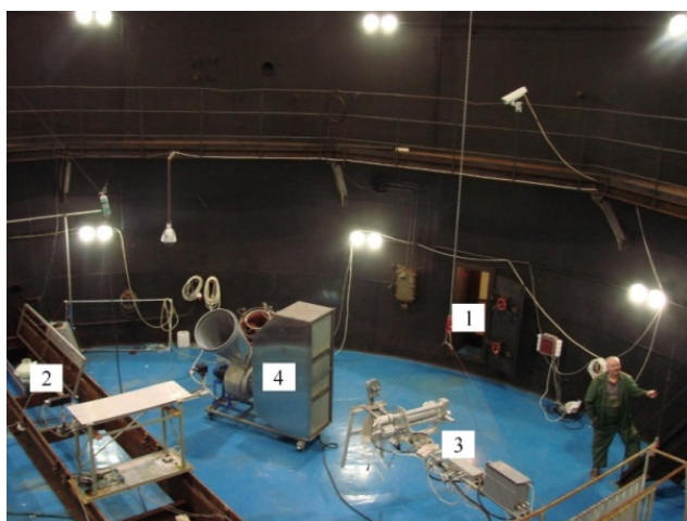
Figure 1. Photo of the LAC interior view. 1—entrance portal with size 60 \times 160 cm 2 ; 2—rail for mounting the tested equipment; 3—the hanging platform with temperature sensors (for measuring dry and wet air), optical depth sensor with 4 m optical path and a photoelectric sensor for measurement of cloud droplets size; 4—inner HEPA filter.
