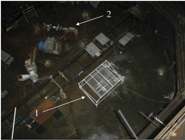
Figure 1. The photo of the placement of the ion wind generating unit in the large aerosol chamber. 1—installation, 2—medium transparency meter based on a helium–neon laser [23] .
