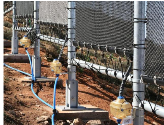
Figure 9. Collection of water droplets, made in the form of a flat mesh [31] .
