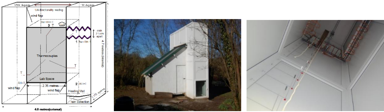
Figure 1. Airflow Measurement under Cooling: (a) Experimental Setup, (b) The Structure, (c) Cooling Coil Configuration ©Peter Bunyard [15,16] .
