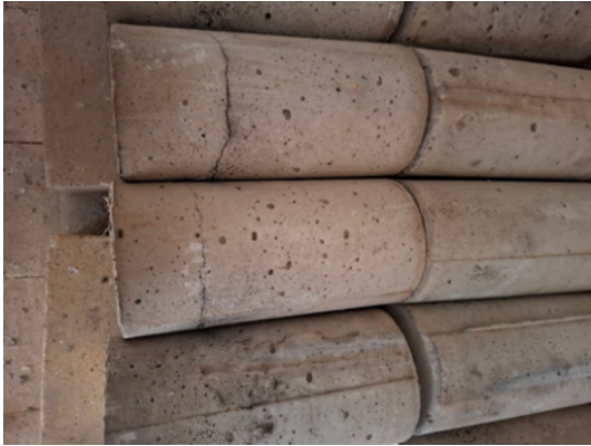
Figure 9. Spalling on the surface of steel fiber-reinforced RPC after burning at 400 °C for 2 hours.
