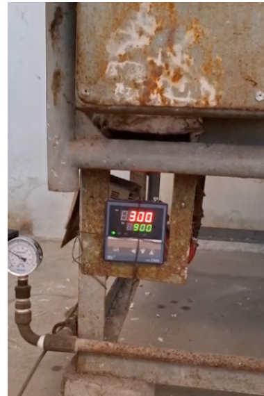
Figure 2. The thermocouple is at a temperature of 300 °C.
