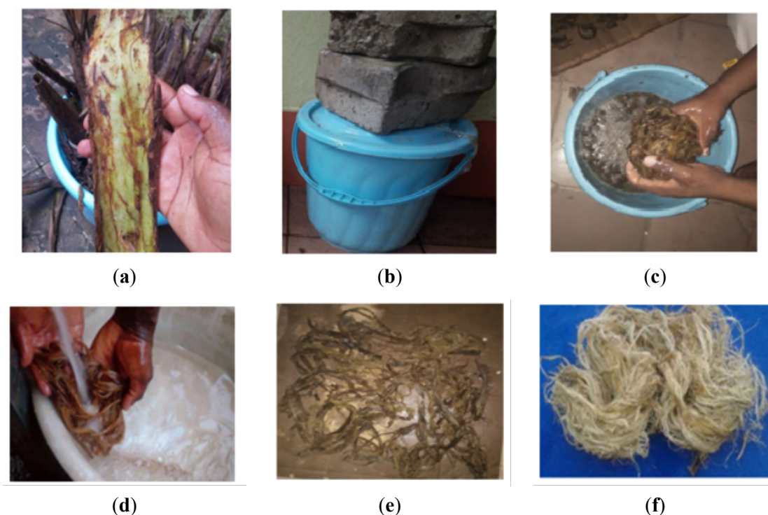
Figure 4. Process of fiber extraction from TP.
