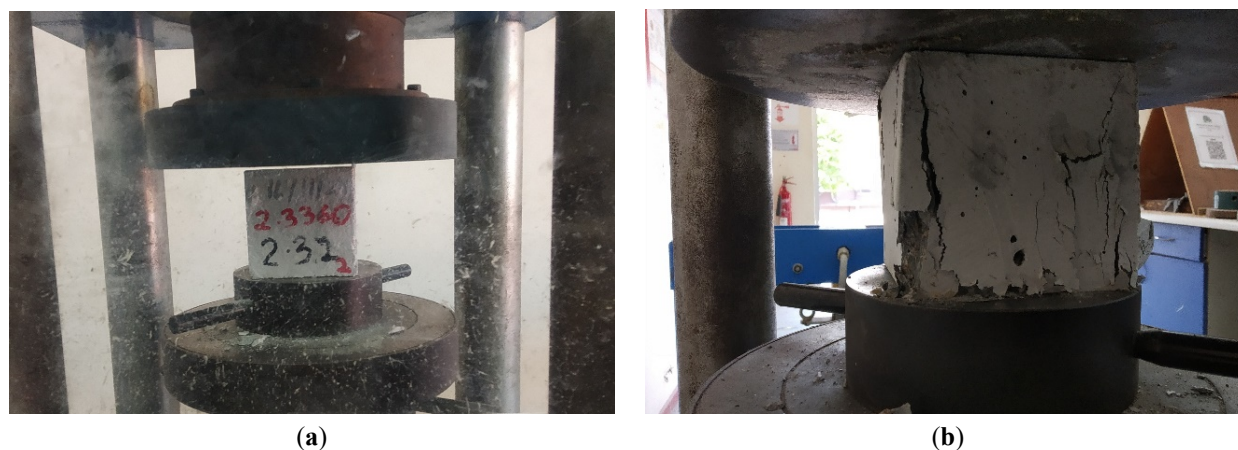
Figure 3. Compressive strength procedure illustrating (a) specimen placement and (b) post-failure condition.
