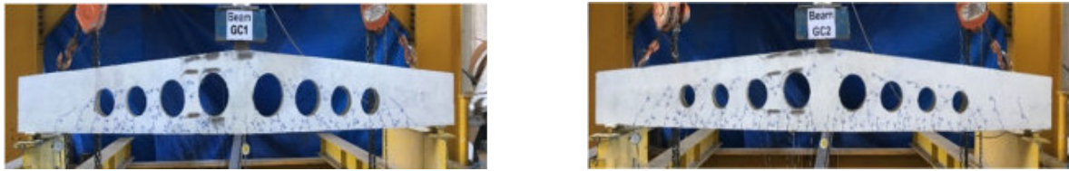
Figure 8. Tested models of reinforced concrete gable beams.
