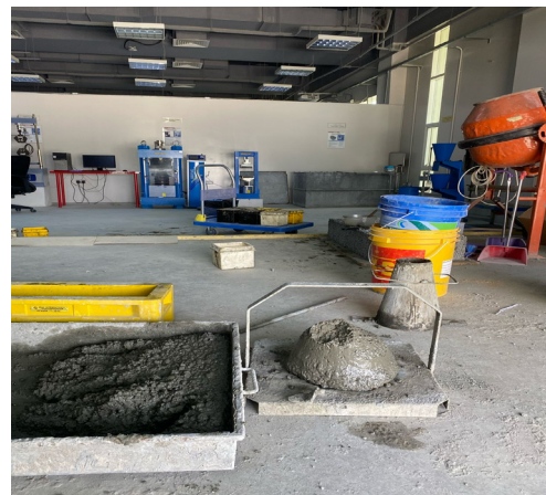
Figure 6. Preparation and testing workability using slump cone apparatus.
