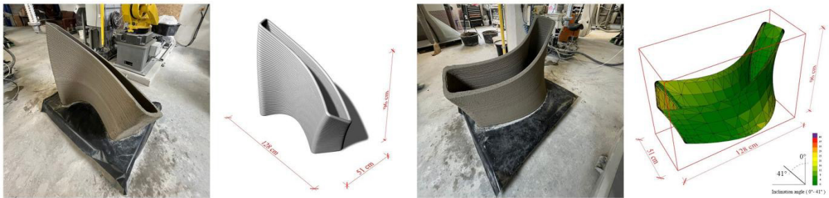
Figure 13. A 3D concrete printed segment from the Cantilever shell, shown in Figure 10 , which validates the capacity of the optimization algorithm to segment a shell into printable pieces.
