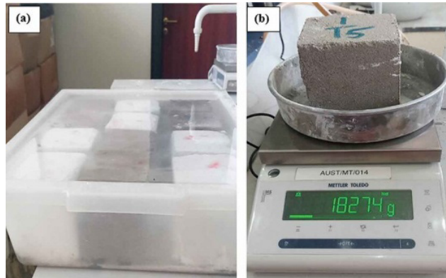
Figure 8. (a) Water absorption test setup; (b) Water absorption sample weighing.
