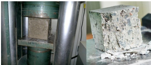
Figure 3. Cube test to check the compressive strength of concrete.
