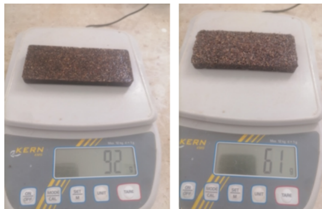
Figure 6. Influence of palm fiber content on the density of composites.
