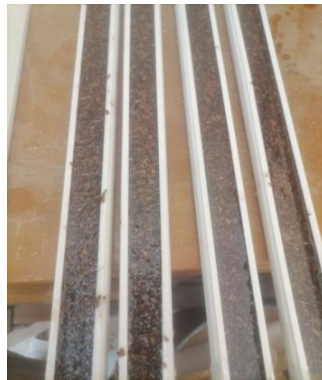
Figure 2. An open-mold casting procedure used for manufacturing the composite specimens.
