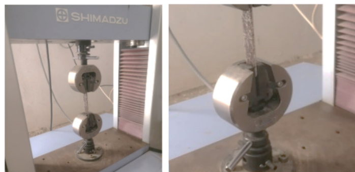
Figure 3. A tensile testing setup used for the evaluation of the mechanical properties of the composites.
