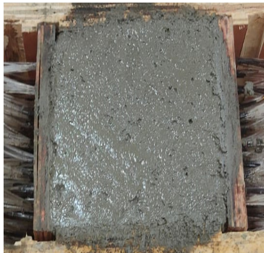
Figure 4. Casting of Concrete Specimens.
