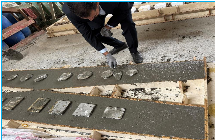
Figure 11. The process of casting specimens of reinforced concrete gable beams.
