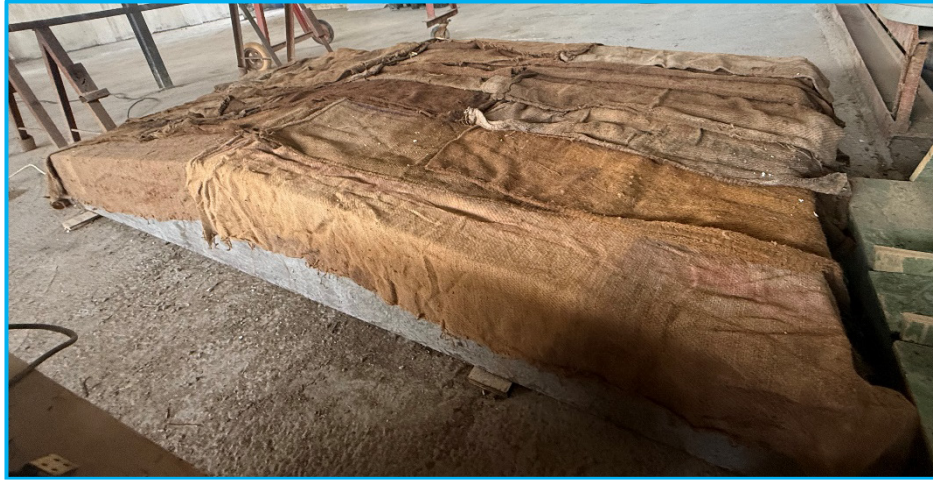
Figure 12. Curing of gable beam specimens.
