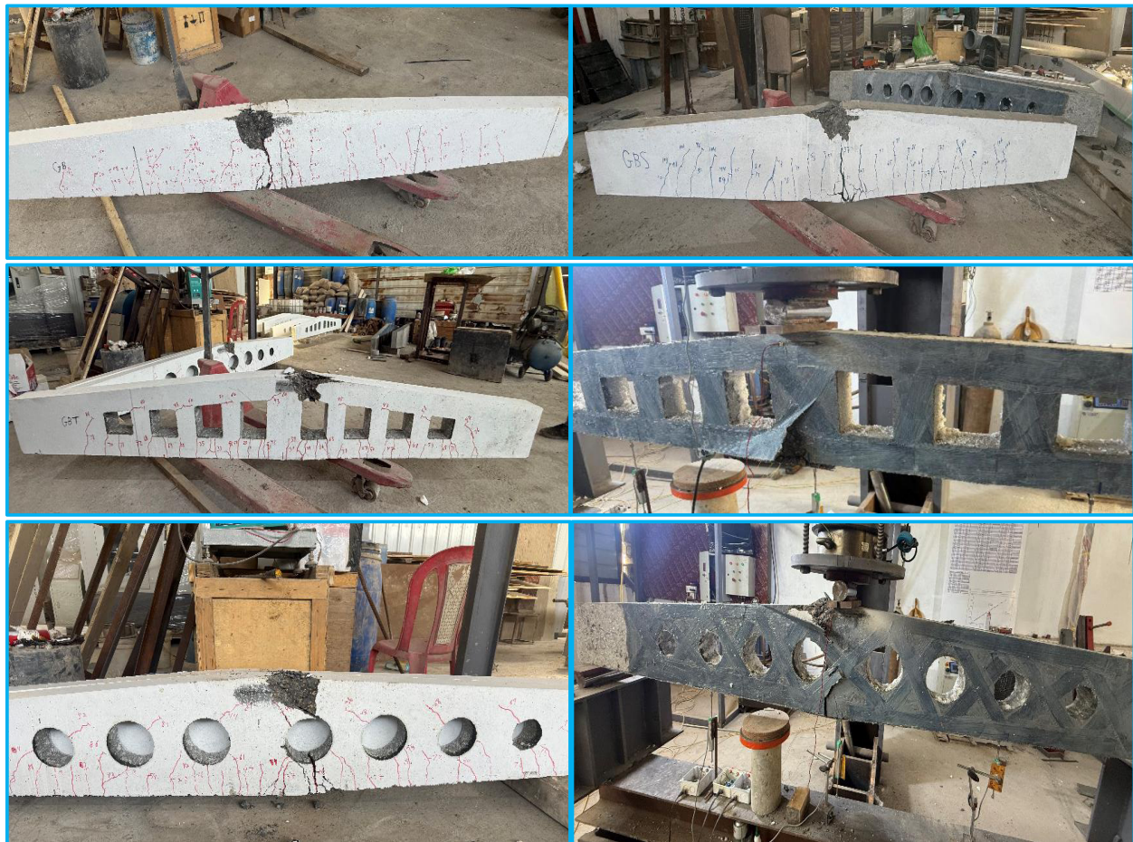
Figure 20. Crack pattern and failure mode of the tested gable beam specimens.
