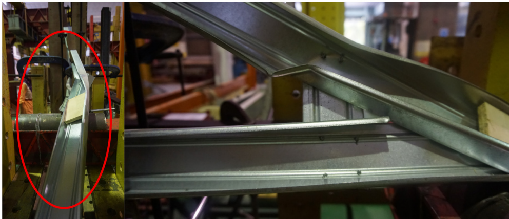
Figure 9. The buckling failure at the bottom and top chords of the CFS channel.
