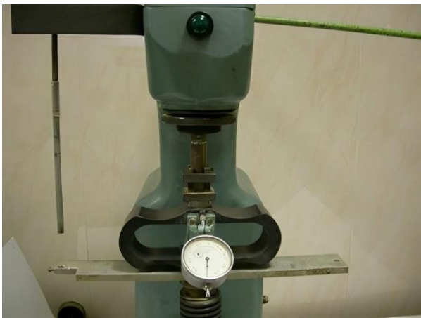
Figure 1. Apparatus for determining compressive strength.
