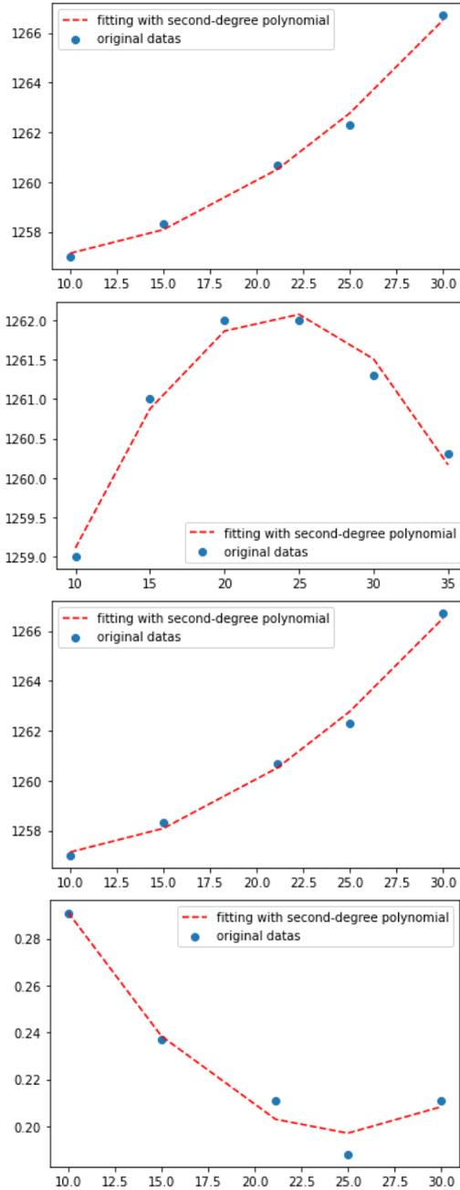
It can be obtained from the analysis of the diagram that when the ratio of powder distribution is 15-25, the assimilation temperature of sinter is higher and the liquid phase fluidity of sintered products is low, that is, the quality of sintered mineral products is relatively high and the energy consumption cost of sintering process is relatively low.
